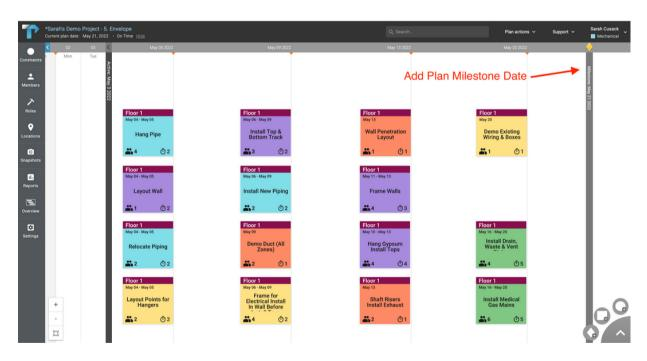
Pull the tickets from the high-level sequencing area into the look-ahead schedule by dragging the Active Line across the tickets. All tickets will have a start and finish date applied to them based on where they are placed in the timeline and will be put into Gantt Bar form. Make adjustments to the tickets as needed and start wrapping up the meeting.
