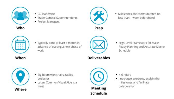
The primary goal of a phase plan meeting is to create a high-level sequence of work that is 'pull planned' backward from the major milestones in the phase. The team collaboratively breaks work down into task tickets to identify handoffs between trades, crew size, and material requirements. This is a loosely structured meeting that works backward from a project schedule milestone and focuses primarily on tasks that release more work.
