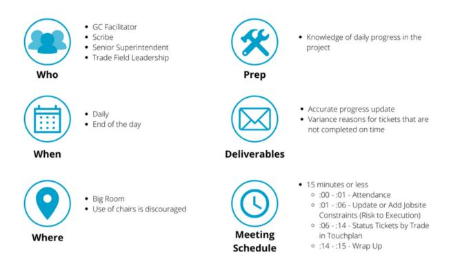
Daily Huddles reinforce teamwork and collect accurate data on job site performance, this is not a coordination meeting. Pinned tickets must be checked daily and be marked as completed on time, early or late. It is here that production data is collected to be made useful later for learning.
